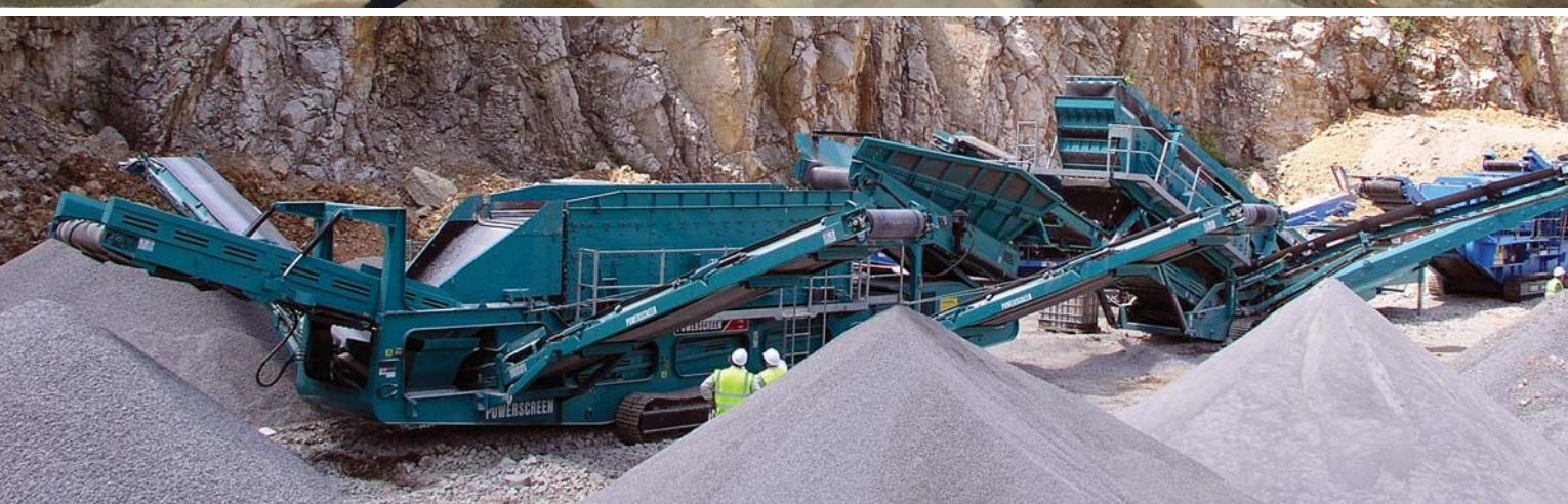
The Powerscreen® H range feature horizontal screens ideal for handling high volumes of sticky materials and for the exact, fine sizing demanded for many construction contracts. Powerscreen® H range is ideal in applications such as natural & crushed aggregate, coal, iron ore, overburden, recycled concrete and asphalt.
