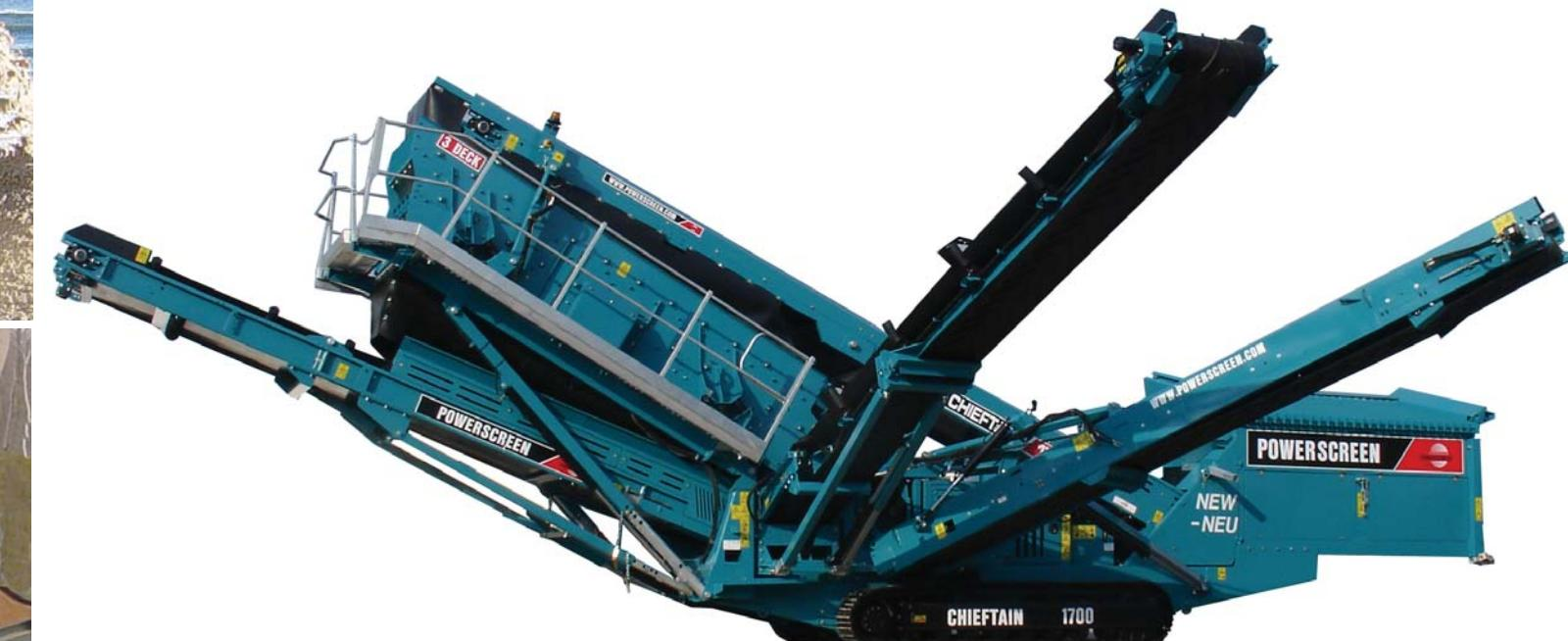
The Powerscreen® Chieftain 1400 is Powerscreen's most popular mobile screening product in the Chieftain range. With proven features such as the patented 4 bearing screenbox, hydraulic screen angle adjustment, user friendly screen access walkways, hydraulic folding conveyors and fully mobile track and wheel chassis configurations. The Chieftain 1400 is the obvious choice for mid-sized operators and contractors in the mining, quarrying and recycling industries.
